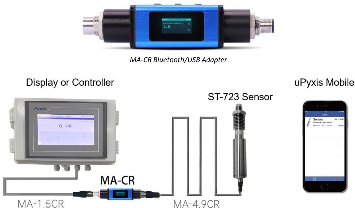
Figure 6. Power the ST-723 via Controller with the MA-CR Bluetooth Adapter inserted between Bulkhead & Flying Lead Cables
