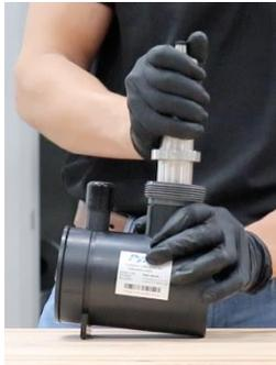
**Tighten Sensor Nut**
