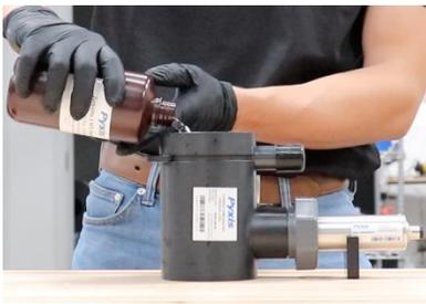
**Insert Lid and Remove Air Bubble Vent Line Cap**
