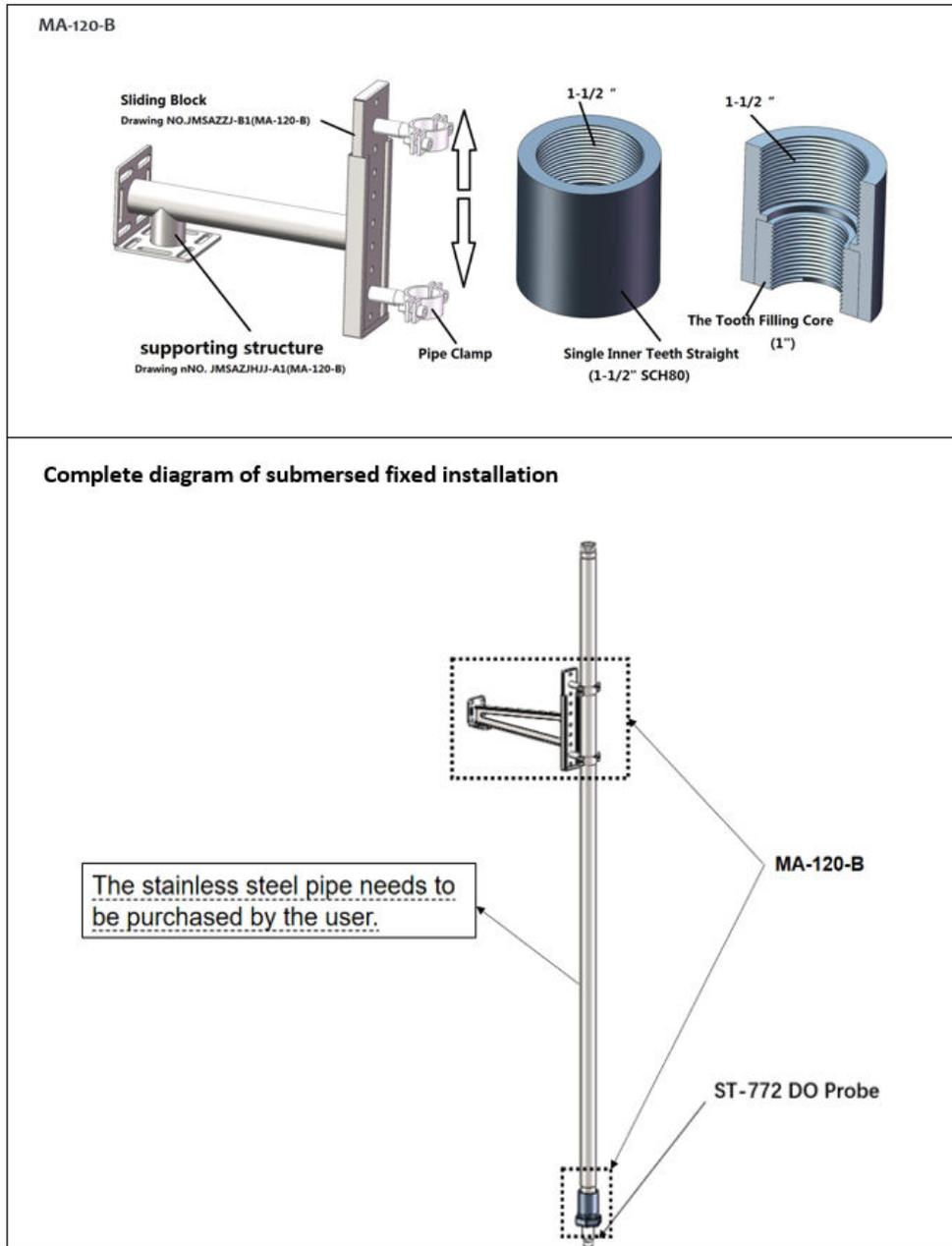
Figure 2. ST-772/ST-772-P in a submersed fixed installation
