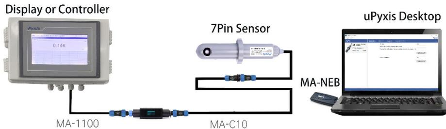
Figure 11. Bluetooth connection to ST-601 sensor with MA-WB and MA-NEB and uPyxis Desktop App.
