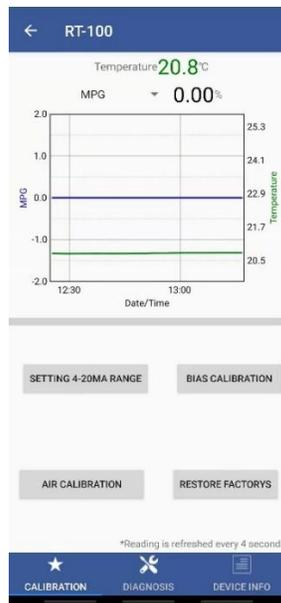
**Figure 26.** – Calibration Screen Interface uPyxis Mobile APP.
