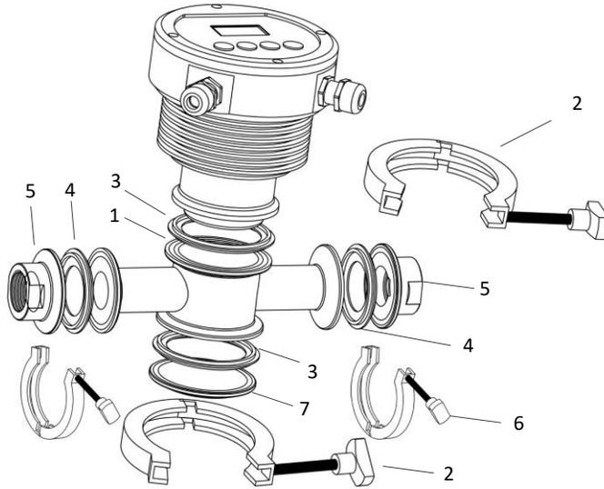
Figure 3. Prism RT-100 Tri-Clamp Flow Cell Assembly (P/N: 56206)
