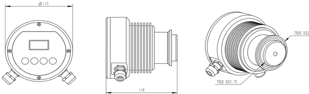
**Figure 2. Prism RT-100 Sensor Dimensions (mm)**
