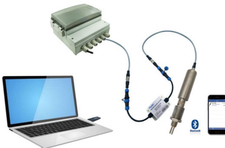
Figure 9. Bluetooth connection to CR-301 sensor
